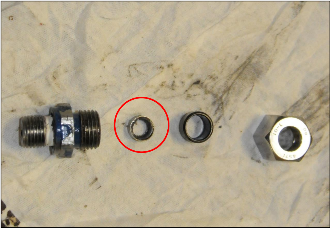
Figure 14: Fitting with broken-off piece of pipe
