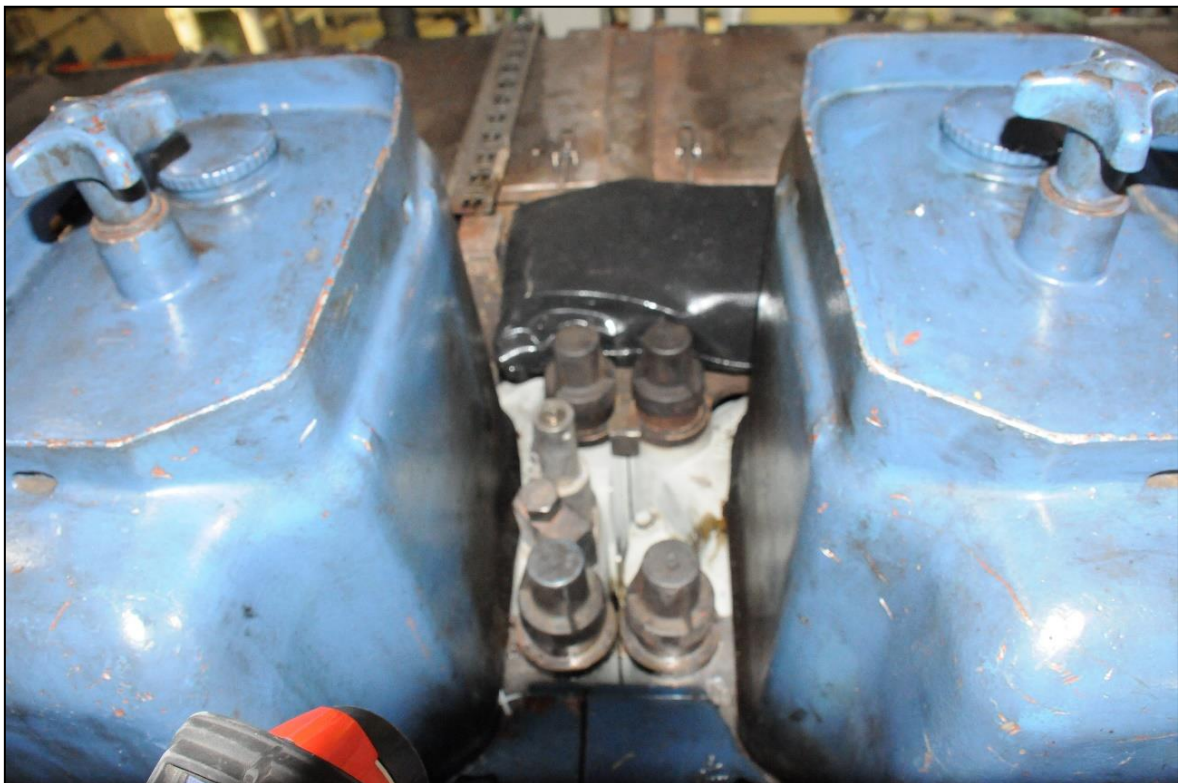
Figure 42: Insulation between cylinder station and exhaust pipe
