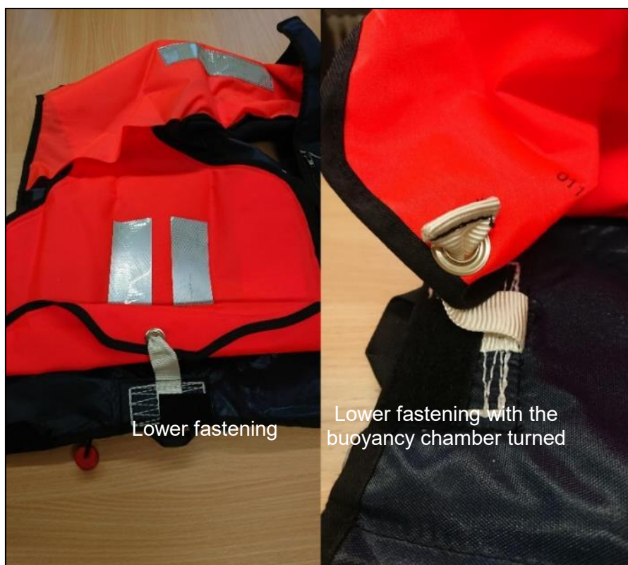
Figure 48: Comparable fastening on a BSU inflatable work vest 128
