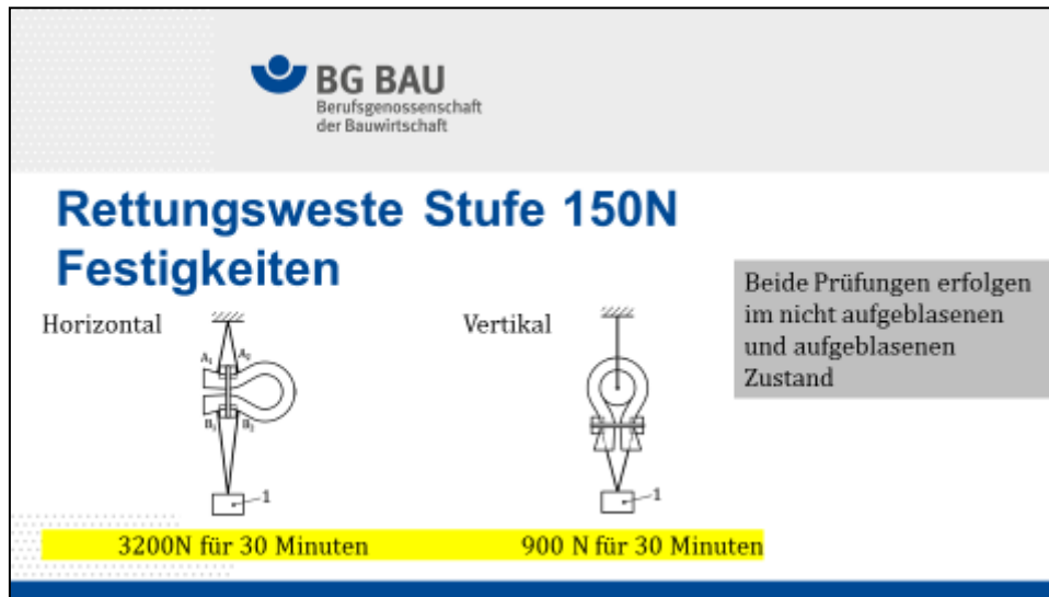
Figure 50: Strength requirements for performance level 150 N lifejackets 135
