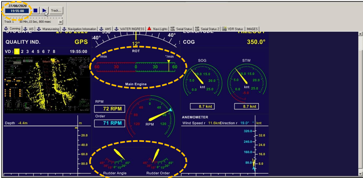
Figure 15: VDR: Hard-over rudder angle and ROT about 30 seconds later (215500 local time)
