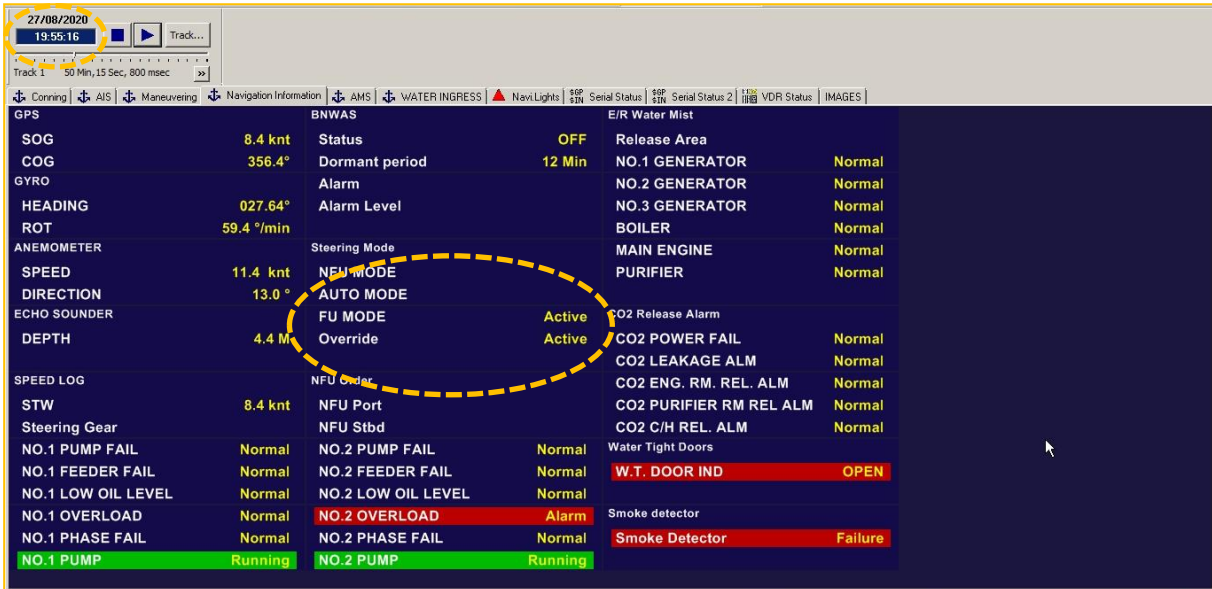
Figure 20: VDR: One second later, 'Override' and 'FU' steering mode still 'Active' (215516 local time)
