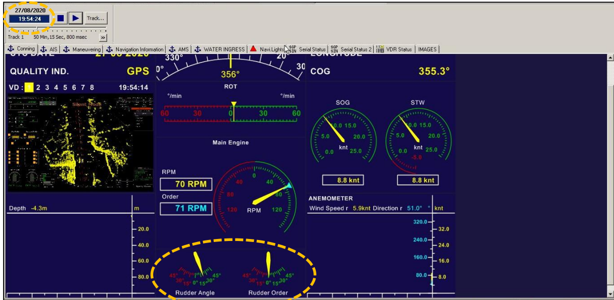
Figure 14: VDR: Non-responsive rudder (first occurrence) 28 (215424 local time)
