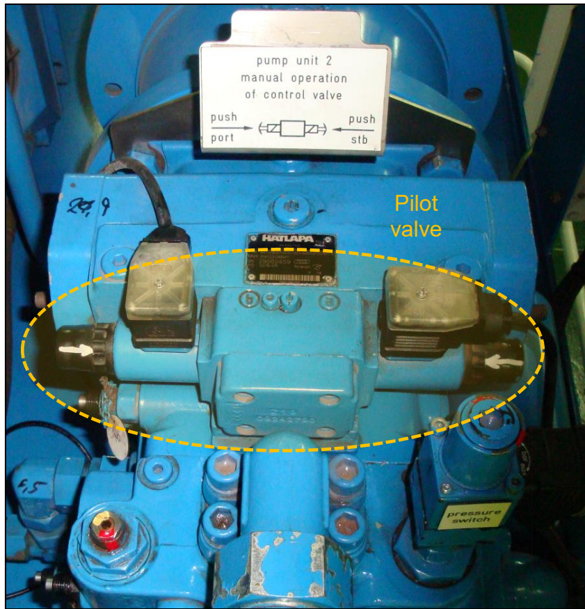
Figure 10: Steering pump 2's pilot valve, incl. brief guide for the emergency control
