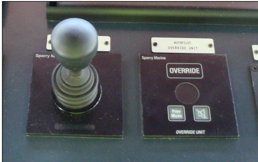
Figure 11: Tiller and Steering Override Unit SOU
