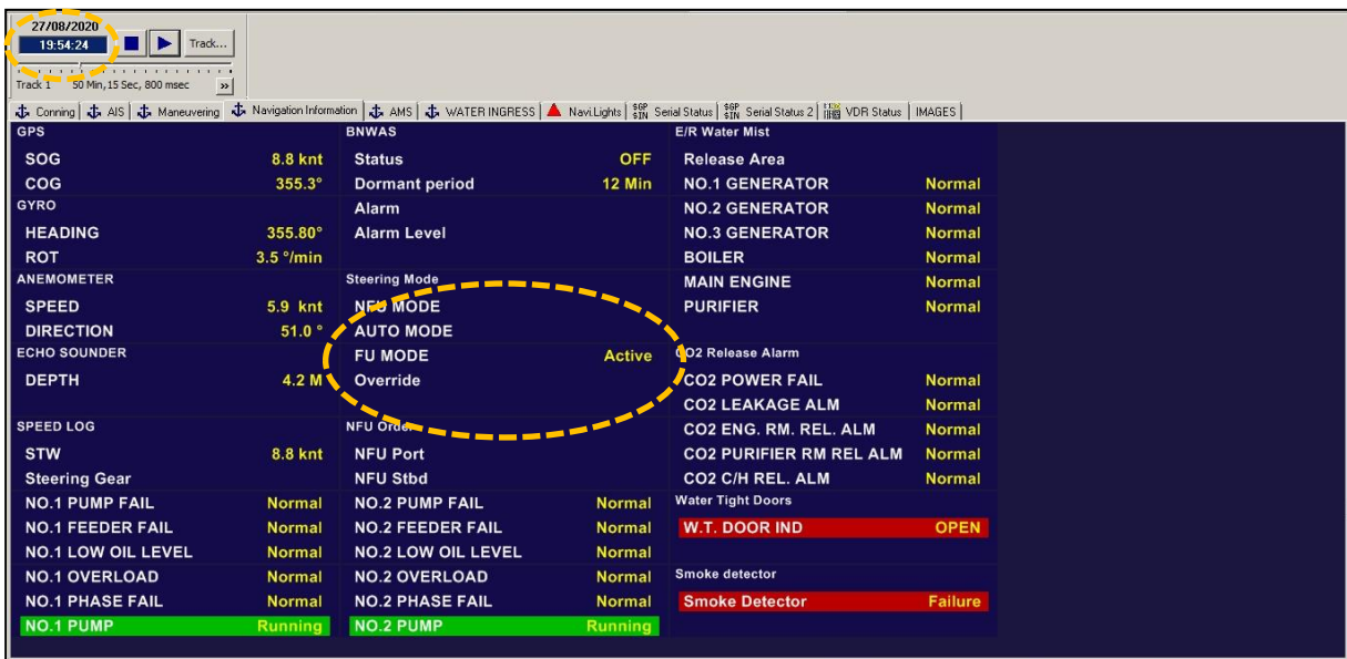
Figure 16: VDR: Non-responsive rudder (first occurrence) (215424 local time)
