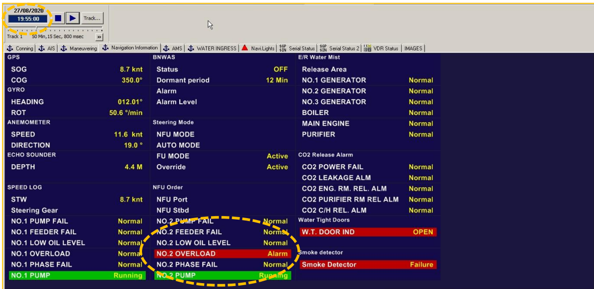
Figure 18: VDR: Steering gear pump alarm (215500 local time)
