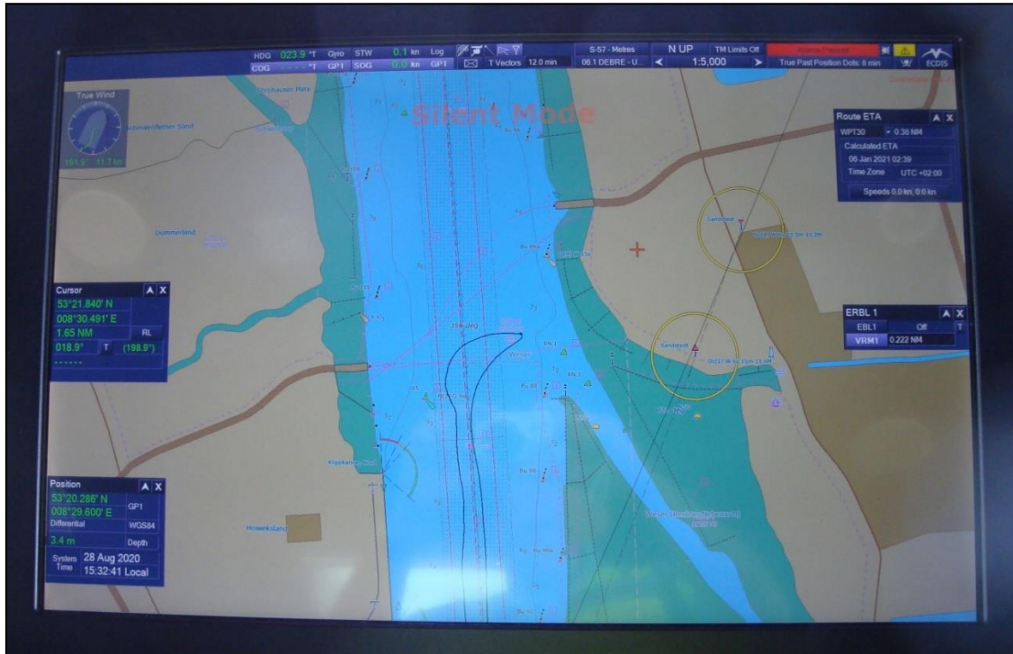
Figure 4: Past track of the accident (RUBINA's ECDIS) 8
