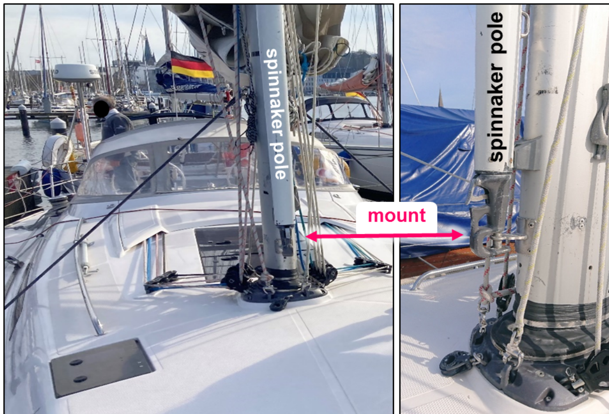
Figure 5: Spinnaker pole attached to the mast where the sheet became entangled 17
