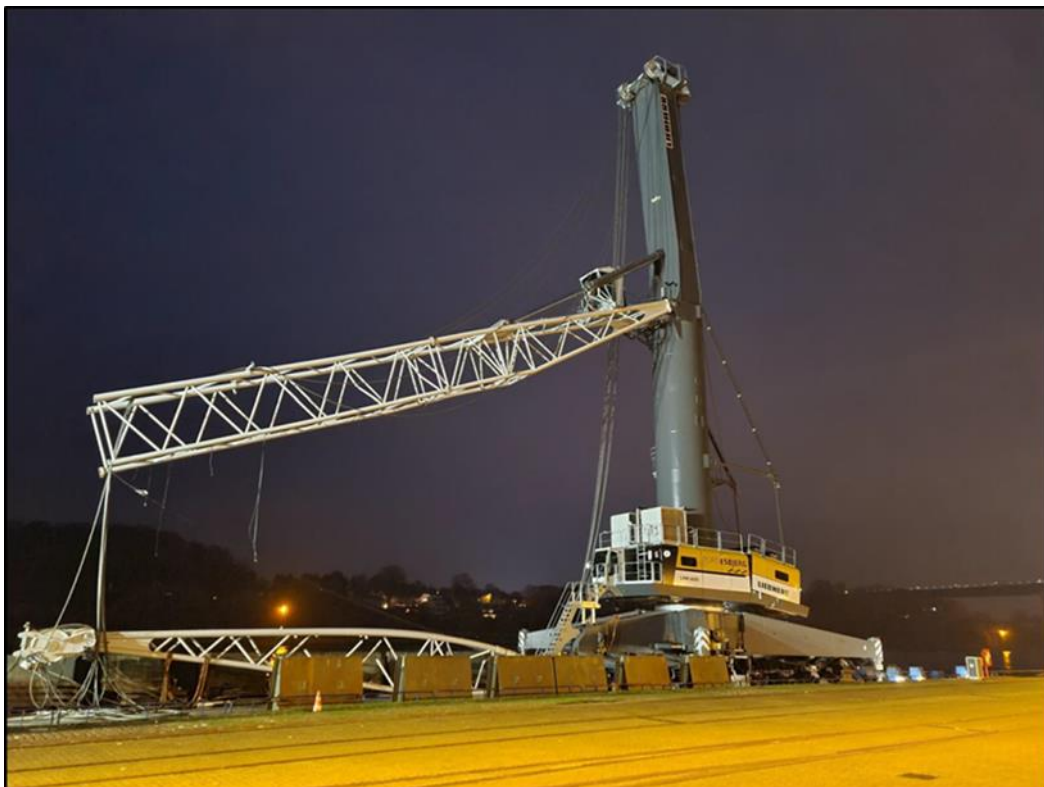
Figure 2: General view of the crane with broken jib 4
