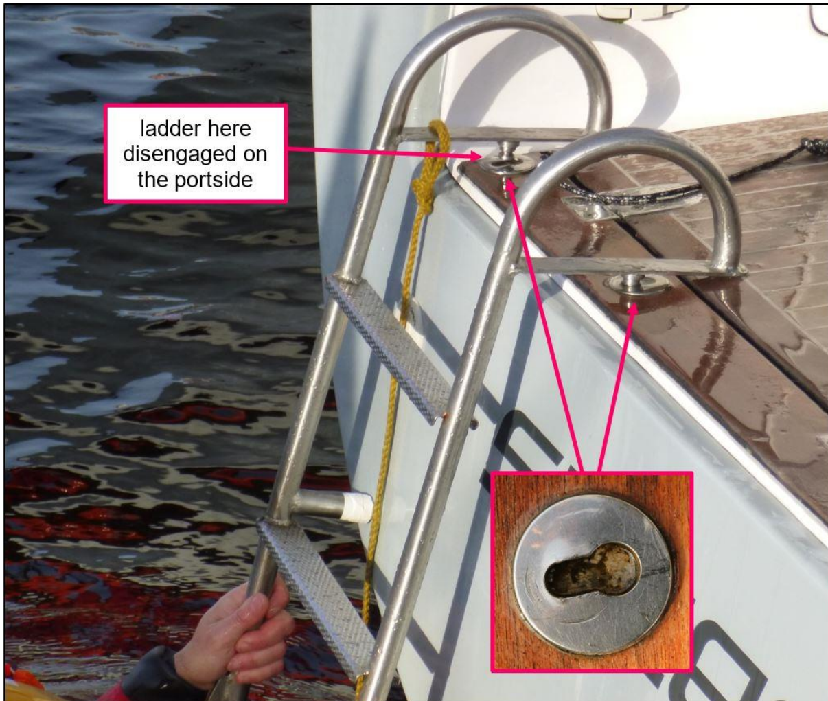
Figure 12: Bathing ladder (reconstruction) SPEEDY GO 32
