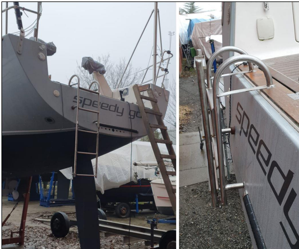
Figure 40: The SPEEDY GO's permanently installed bathing ladder after modification 134
