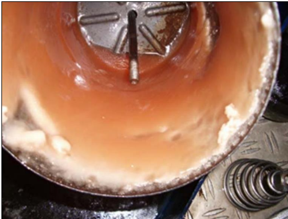
Figure 15: Filter clogged with solidified wax 57
