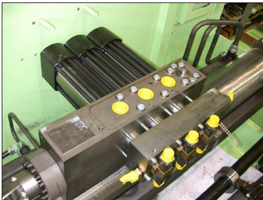
Figure 20: Photograph of an ICU 74 (during installation; various openings still covered with yellow plastic caps.)
