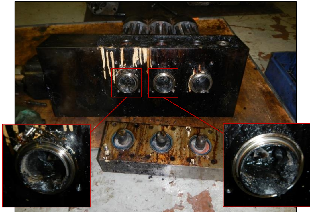
Figure 7: 'Neutral spaces' of an ICU clogged with a tar-like substance
