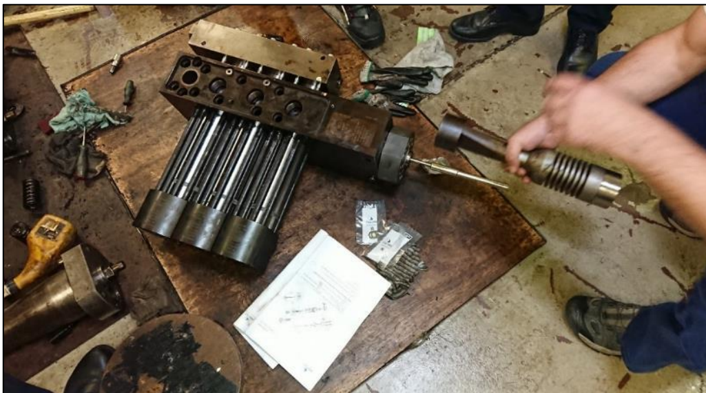
Figure 6: Removed and disassembled ICU with the three injection control valves (left) and the fuel quantity piston (in hand)
