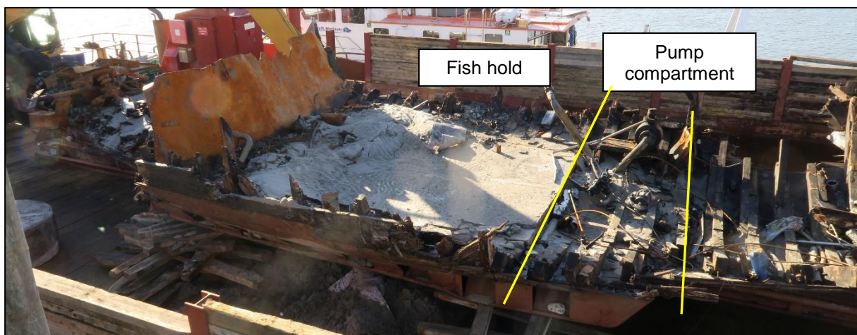
Figure 14: Fish hold and pump compartment
