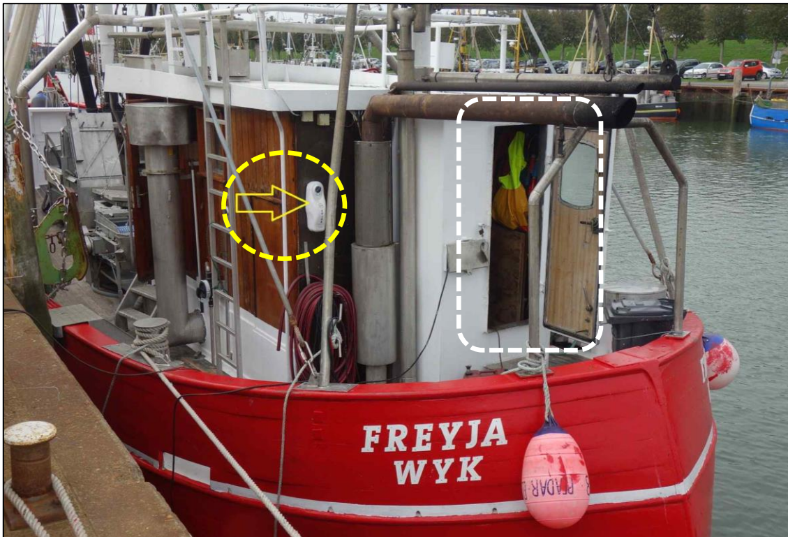
Figure 4: Access to the engine compartment in the aft section of the FREYJA's deckhouse and installation position of the EPIRB 12
