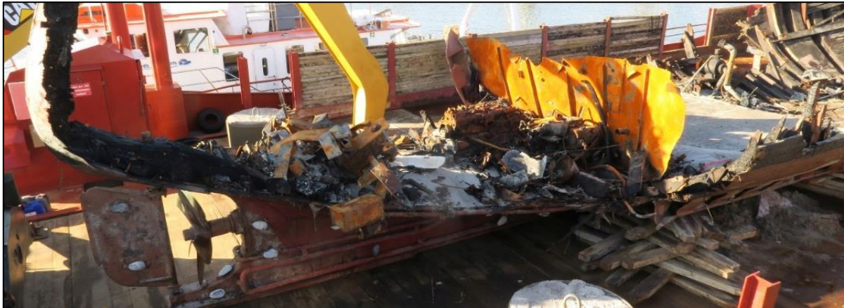
Figure 9: Burnt out wreck of the fishing vessel FREYJA on the deck of the CATJAN (in this case, the vessel's aft section with propeller and remnants of the engine compartment)
