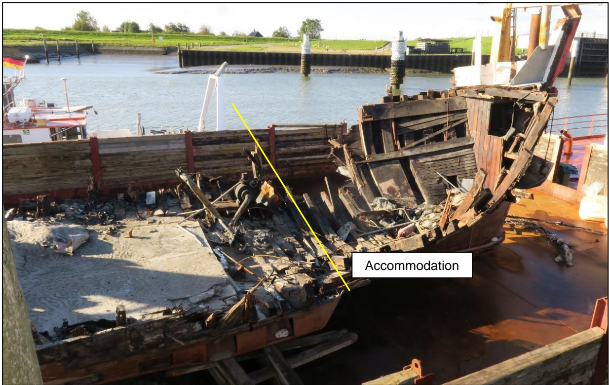
Figure 15: Fish hold, pump compartment and accommodation
