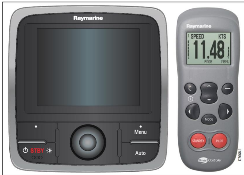
Figure 6: Autopilot Control Units on the SANTA CECILIA 9
