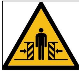
Figure 7: Warning sign W019: Crushing by Moving Parts 10
