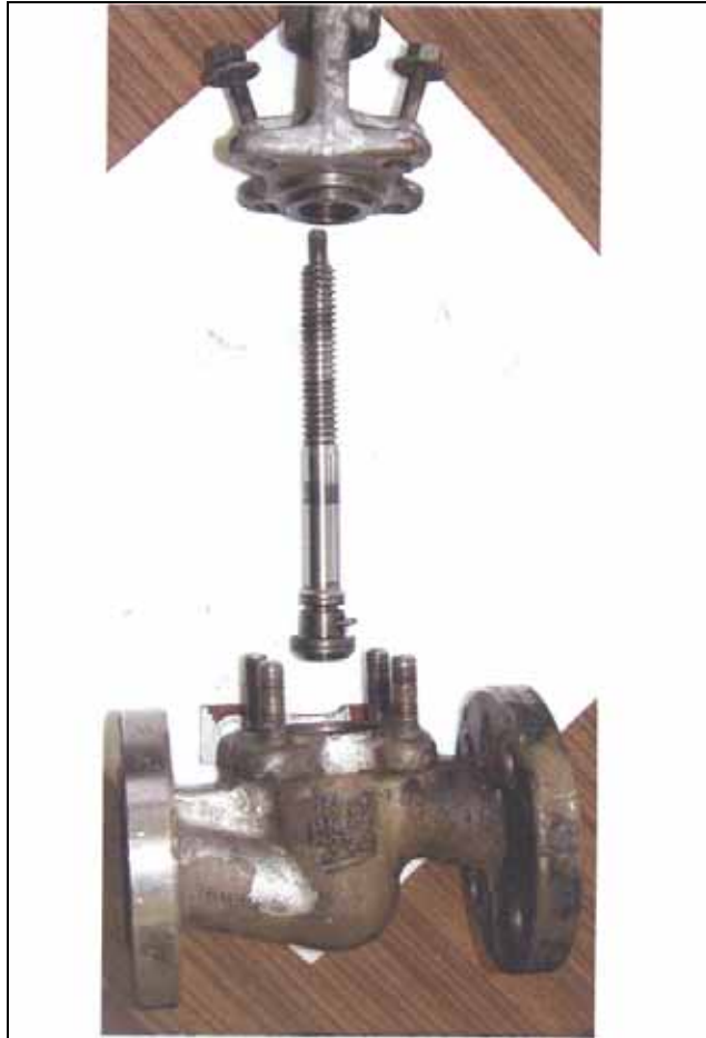
Figure 9: Valve in dismantled and cleaned condition
