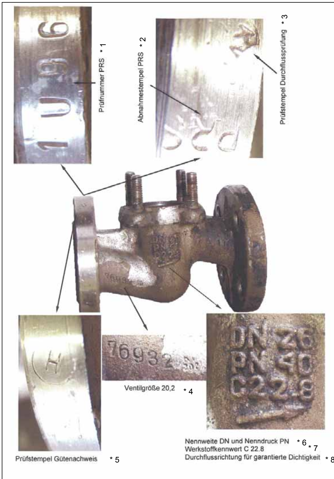
Figure 10: Markings on the valve
