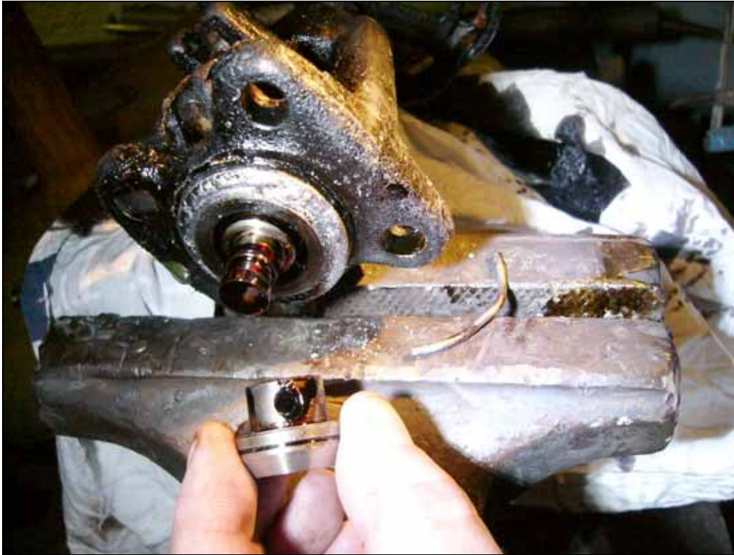
Figure 6: Wire removed and cone drawn off
